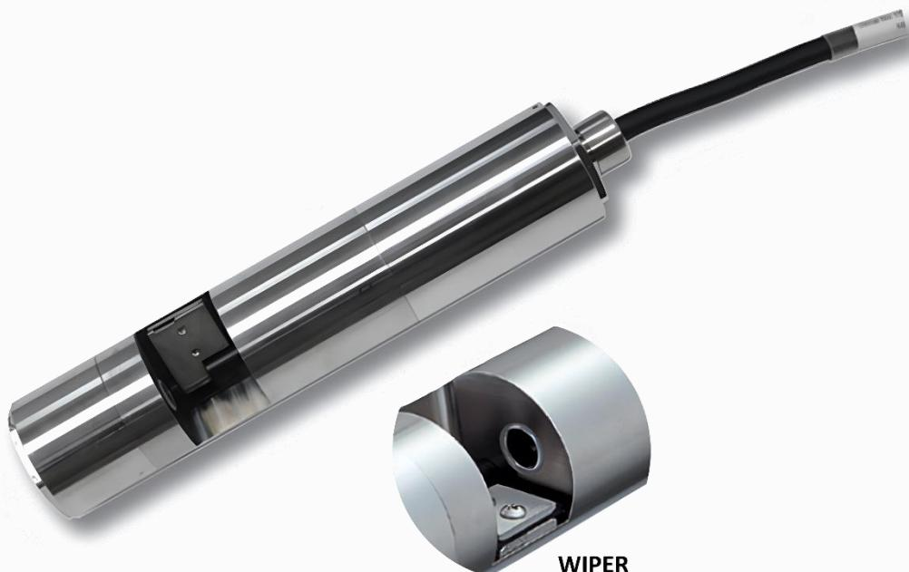
The TC Series Turbidity Sensors have compact design that makes it possible to install these sensors at any place easily. The sensors with different sensing range have built-in analog output function of 4 to 20 mA. This sensor have a built-in wiping cleaning system that keeps the lense clean. These probes are waterproof and can be submerged completely so they are ideally suited for pure measuring tasks in wastewater & effluent measurements.
